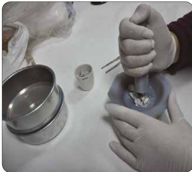
Figure 4: Sample Crushing in Agate Mortar / Örneklerin Agat Havanda Ezilmesi
